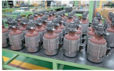
▲ T-rotor pump 조립 Line
