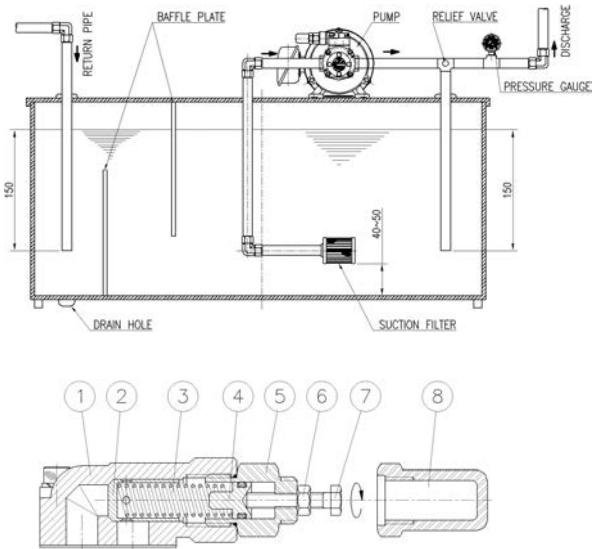
① Relief valve ② Piston ③ Spring ④ Spring seat
