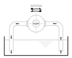
Suction and discharge by rotation direction 회전방향에 의한 흡·토출구
