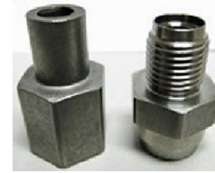
↑ Parts made by cold-forging method
