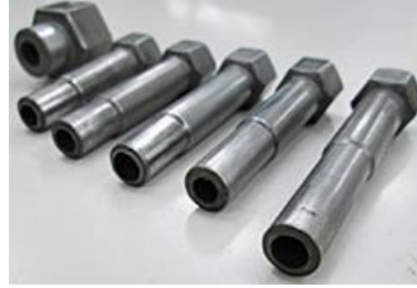
↑ Parts made by cold-forging method
