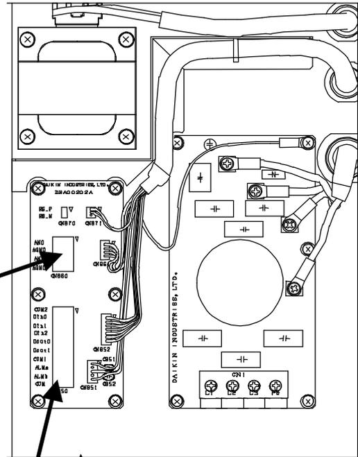
I/O signal cable connection terminal block
