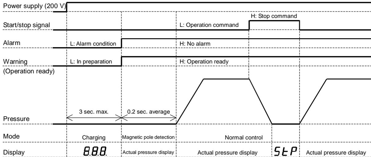
2-2 When the pressure switch function is used
