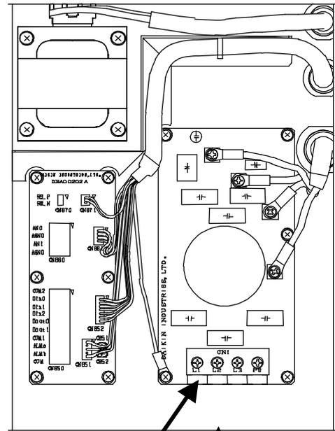
Power supply connection terminal block      Wiring hole
