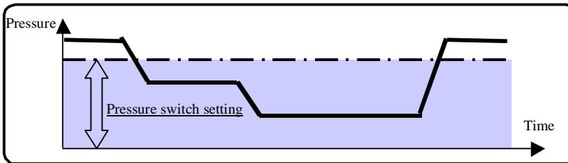
**P18 = 2 (Expansion of pressure switch function)**
