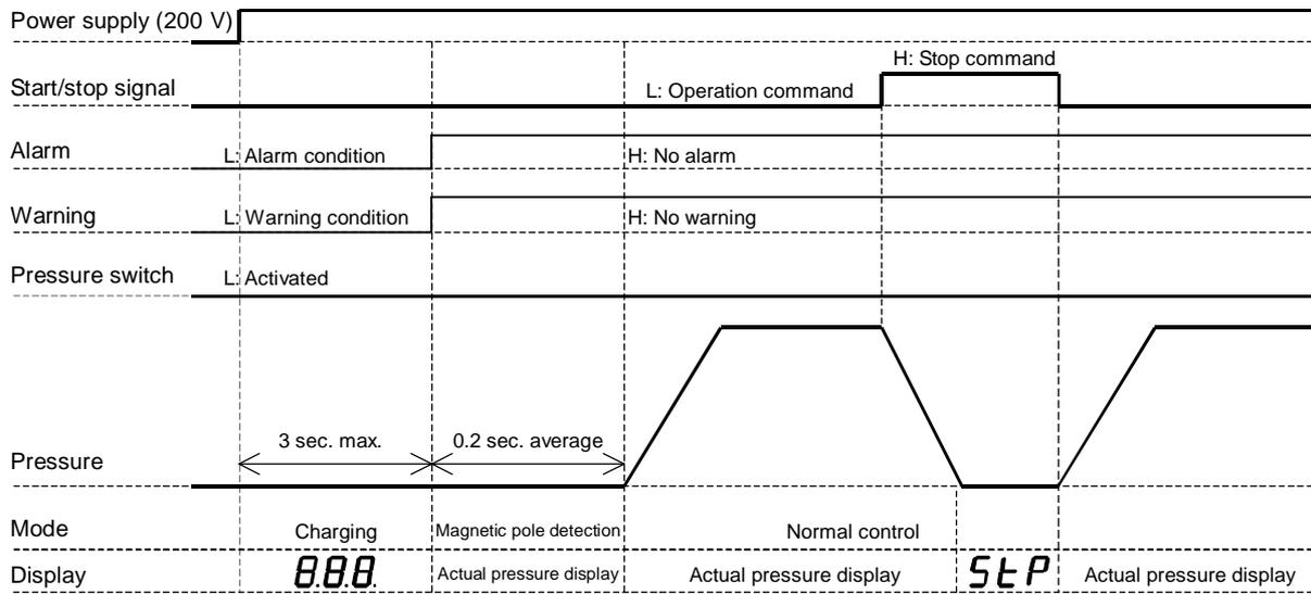
1-2 When the pressure switch function is used
