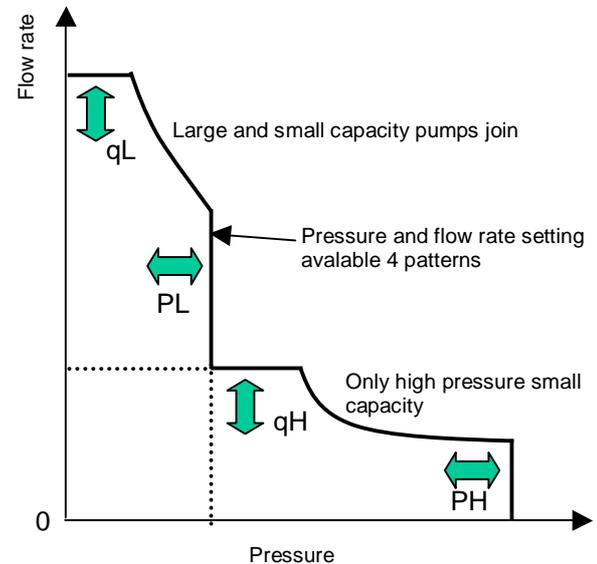
(2) Multi-stage speed control/Multi-stage pressure control, and shockless control functions
