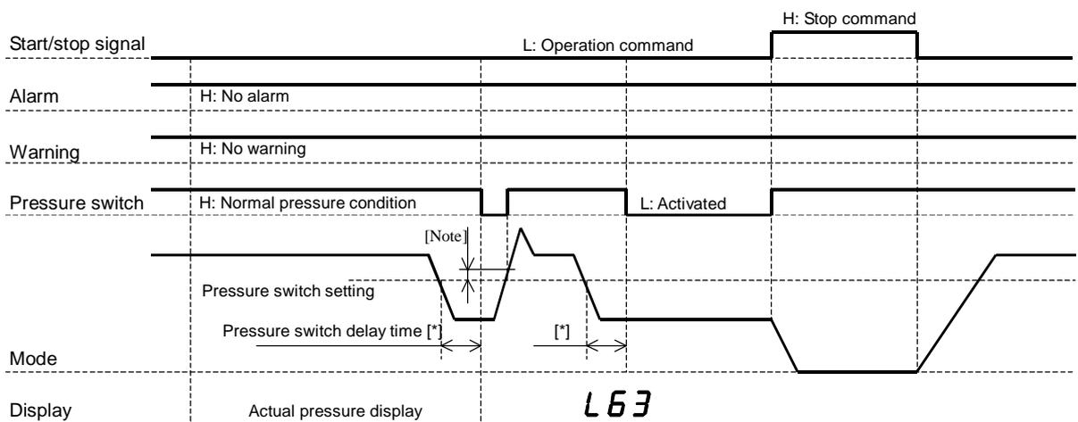
The above chart shows the case where “P08” (Pressure switch display hold setting) is [1] or [2].
