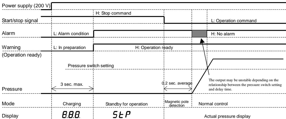
\* Magnetic pole detection will be executed at the first motor startup after power-ON.
