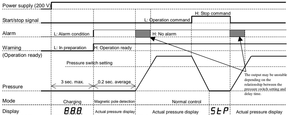
2-3 When the pressure switch function is used (Stop at power-ON)
