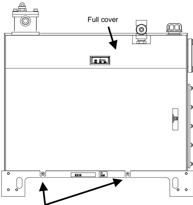
Cross-recessed truss head machine screws
