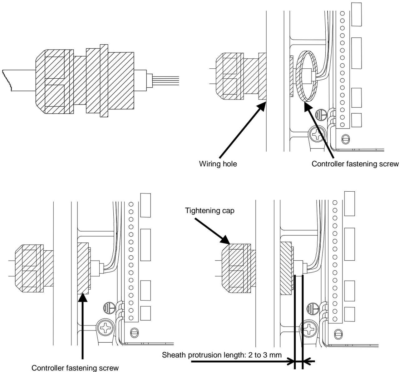
◆ Connecting the main power supply cable
