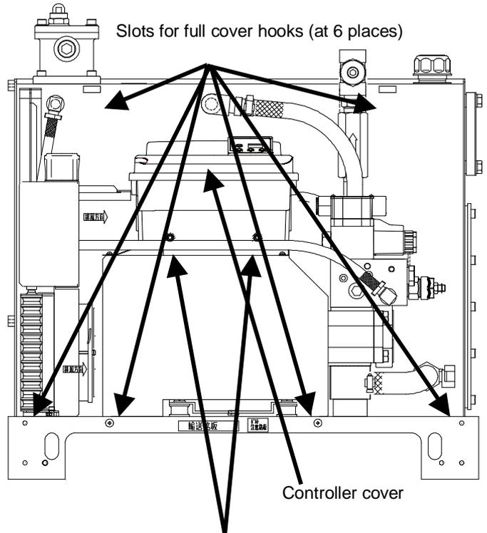
Hexagon socket head bolts for fastening the controller
