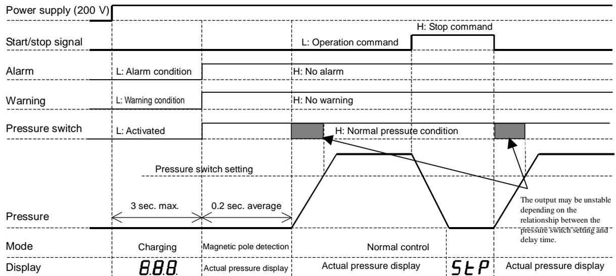
1-3 When the pressure switch function is used (Stop at power-ON)
