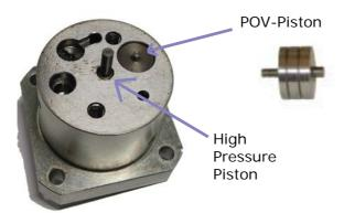
Ensure the high pressure piston is moving freely in the top part. <u>If not</u> return unit to factory for repair.
