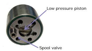
Ensure the low pressure piston and the spool valve are moving freely in the housing. <u>If not return unit to factory for repair</u>.
