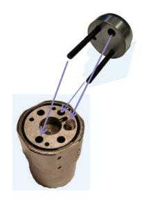
4.4 Position the intensifier housing parts on top of of the block positioned as shown, and tighten the 2 off M6 x 100 screws with a torque of 18 Nm,
