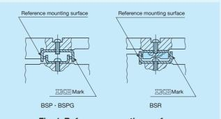
Fig. 1 Reference mounting surface
