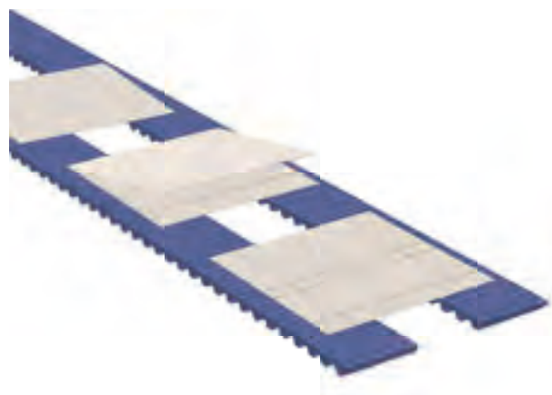
Figure 6.6.2: Vacuum-supported parallel conveyor for paper
