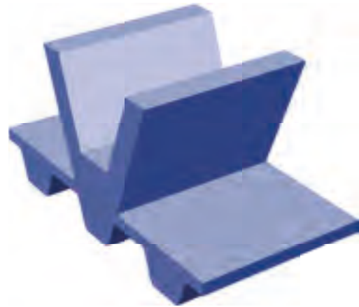
Figure 6.4.14: Optimum cleat position directly opposite the belt tooth
