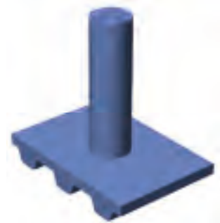
Figure 6.5.3: Cylindrical round cleat: standing cylinder
