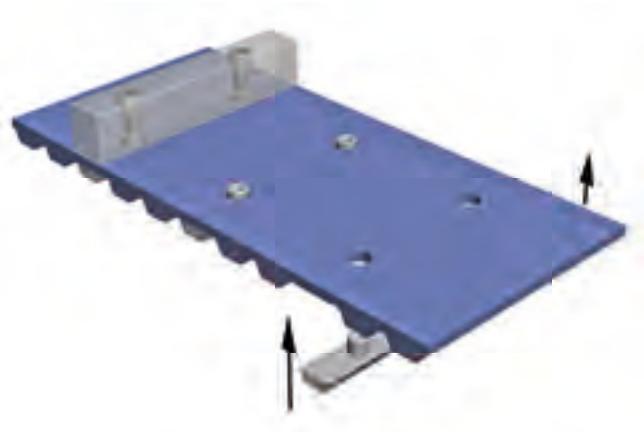
Figure 6.4.16: Installation of metal tooth and screwed-on cleat
