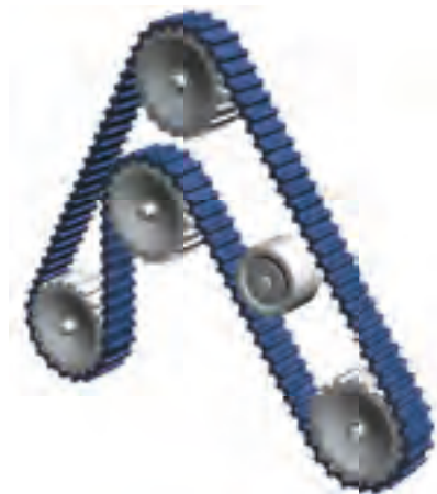
Figure 3.2.2: Multi-pulley drive with inside, smooth cylindrical pulley
