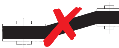
Axial misalignment of pulleys
