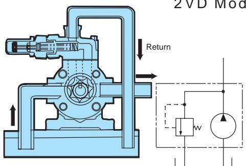
This relief vale is used in the same manner as the above , but it can also be directly attached to the Trochoid pump 2HB model.
