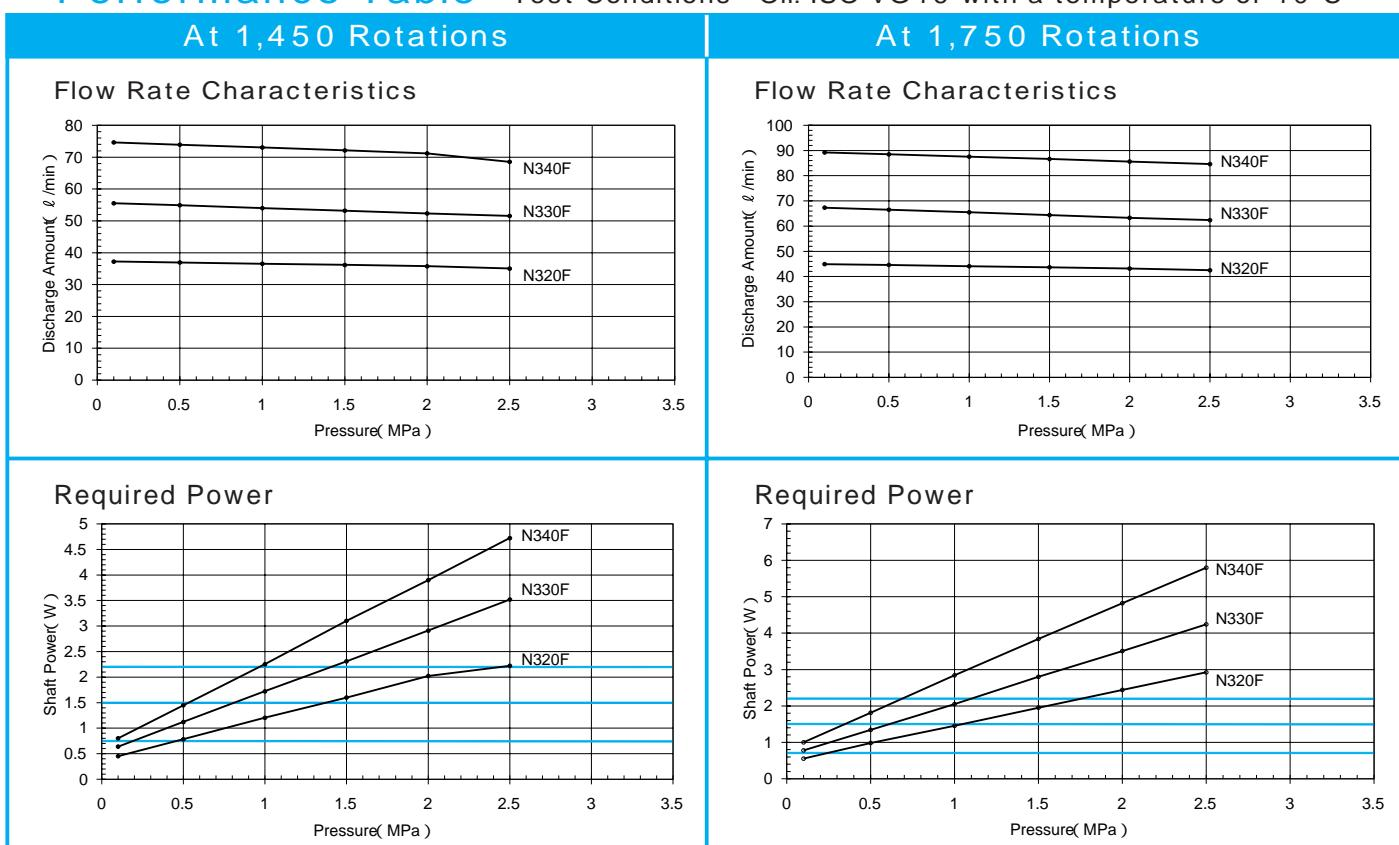
Select the best motor using the lines in the "Required Power" table as the applicable standards.
