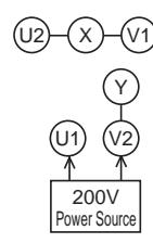
U2-Y-V1 in the clockwise direction as seen from the pump side
