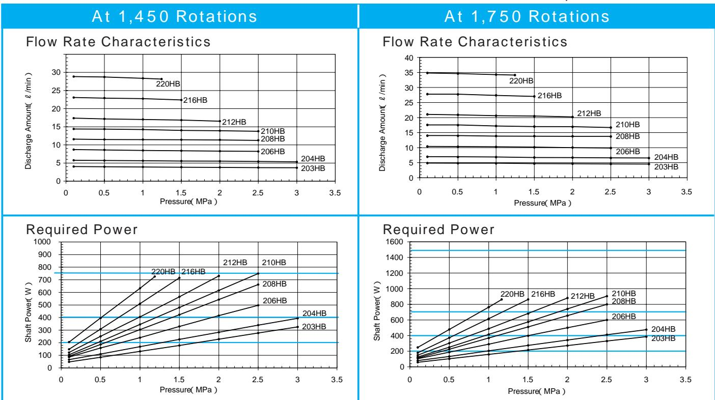
Select the best motor using the lines in the "Required Power" table as the applicable standards.
