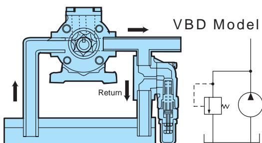
This method uses adjustment valves (valve and sub-plate) to regulate the oil pressure (or for forced circulation).
