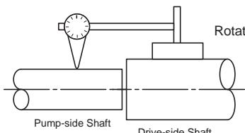
Rotate the dial gauge 360 ° and set so that the dial gauge run-out is within 0.05mm.
