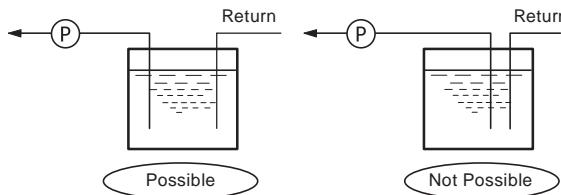
Piping on the suction side should be as short as possible and with the smallest number of curves possible.
