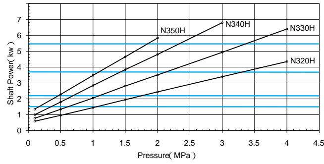
Select the best motor using the lines in the "Required Power" table as the applicable standards.
