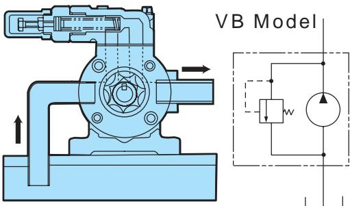
With this method the valve is connected directly to the pump to momentarily lower pressure when the oil is being transmitted.
