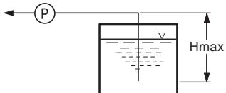
Keep the suction-side piping as far away as possible from the return port of the relief valve or actuator so that there will be no negative influence from the returning oil.
