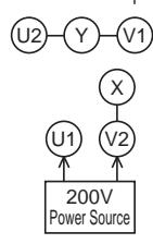
Counter-clockwise seen from the pump side
