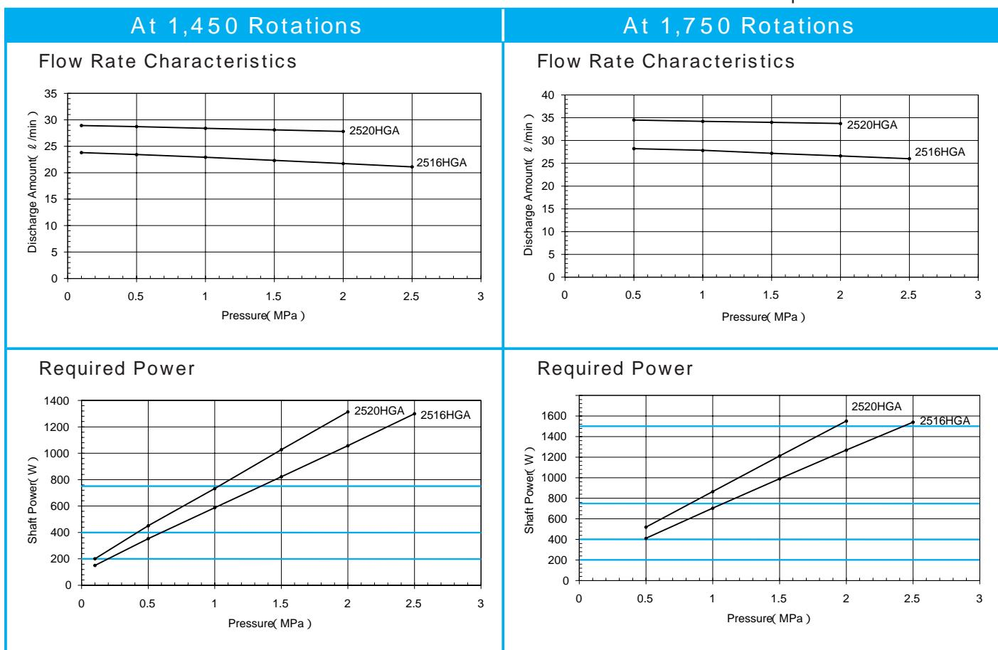
Select the best motor using the lines in the "Required Power" table as the applicable standards.
