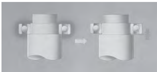
● Figure 9.3 Shaft Shoulder Gap After Cooling
