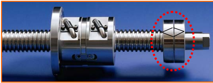
V mark is pointing in the direction of the load (in the application) applied to the outer ring.
