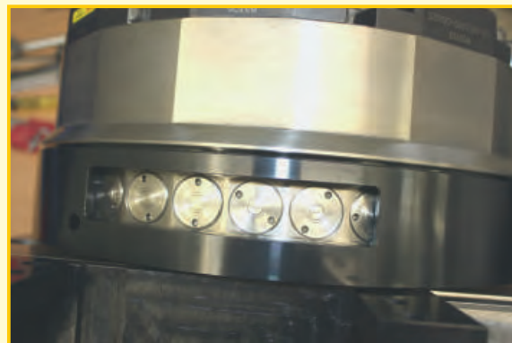
(2) Coupling nipples in the revolver fixture (with a total of 36 coupling nipples)
