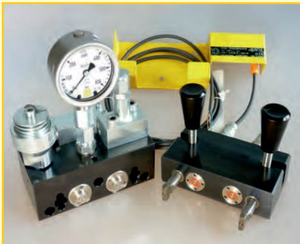
Double-acting coupling nipple unit with 13 cm 3 hydraulic accumulator (l.), coupling mechanism board (r.) and safety holder for coupling mechanism board with proximity switch (b.).
