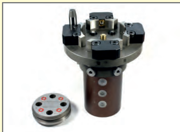
4-fold coupling system with hydraulic clamping, coupling nipple plate with glow jet, combined with 6-lead rotating bush NW5, can be coupled without pressure (left) coupling mechanics plate
