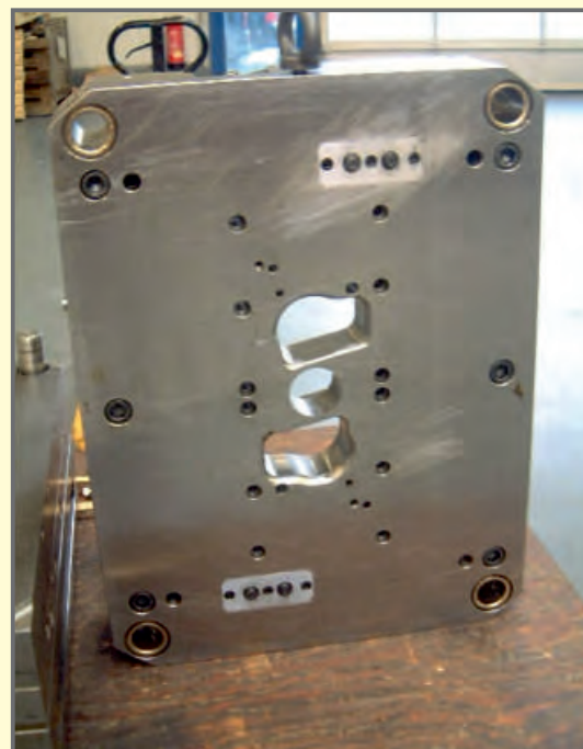
Front tool plate, rotation-symmetrical positioning of coupling nipples for 0° - respectively 180° setting
