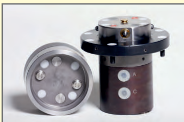
2-fold coupling system with hydraulic clamping, flow jet and 4-lead rotating bush, coupled without pressure
