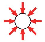
The patent pending Z-Lock is the first ever tapered bore locking collar system. Just tighten the cap bolts properly and the specialized tapered bore collar provides extreme holding power on the shaft without causing any damage. This is a true 360 degree locking mechanism.
