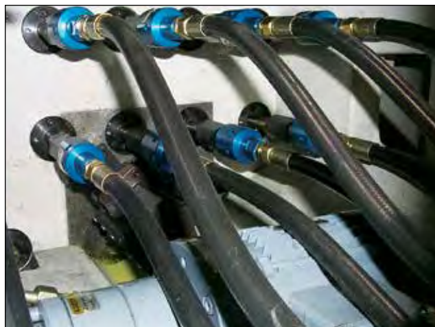
DEUBLIN 1116 Bearing-Supported Unions on Automotive Transfer Line
