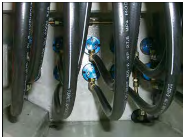
DEUBLIN 1117 Bearingless Unions on Automotive Transfer Line
