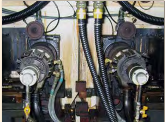
DEUBLIN 2-passage Unions on CNC Turning Center
