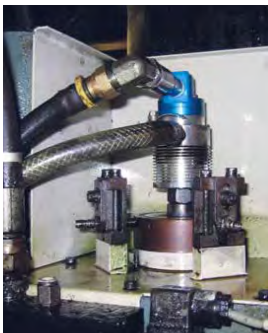
DEUBLIN 1109 on vertical machining center
