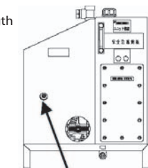
High-pressure safety valve adjusting window
