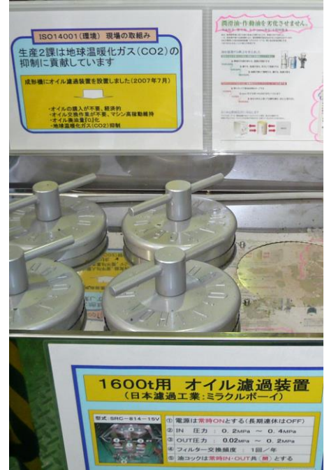
↑Miracle Boy SRC-812-6V & SRC-814-15V installed to injection molding machines manufactured by Toshiba-Machine
