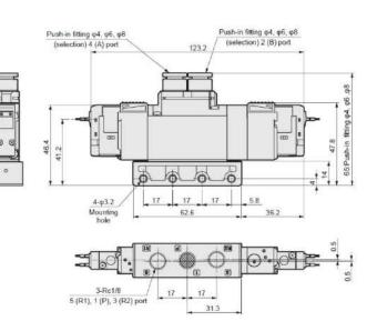
Shown: CKD 4GA24R double solenoid 3-position valve with 'grommet' wiring where flying leads are hard-wired to solenoids.
