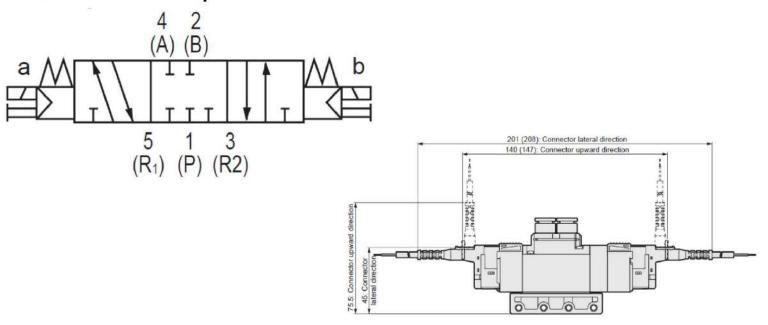
3-position double solenoid valve with cylinder ports connected to exhaust
