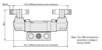
Shown: CKD 4G2B25R double solenoid 3-position valve with DIN connectors.
