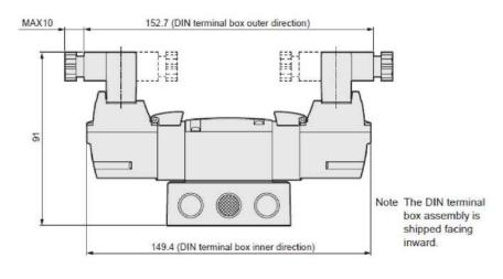
Shown: CKD 4GB220R double solenoid valve with DIN connectors for both solenoids. All ports are on valve sub-base. Shown: Threaded inlet pressure port and 2 exhaust ports.
