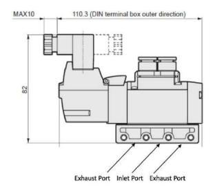
Shown: CKD 4GA210R single solenoid valve with DIN connector and quick-connect cylinder ports coming from the valve body.
