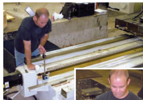
Machine tool calibration of linear axis using laser measurement system
