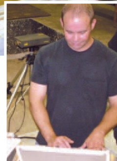
Machine tool calibration of linear axis using laser measurement system
